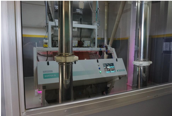
Photo 6.5 State of the art technology a Sortex B camera sorting filter from Bühler
